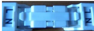
Location of the lock on the connector
