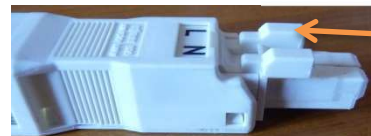
Location of the lock on the connector
