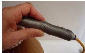
5- Hold the BulM spring with your hand and turn the other part of the spring clockwise. Pull lightly to check for
