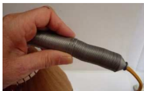
5- Hold the Volupte spring with your hand and turn the other part of the spring clockwise. Pull lightly to check for
