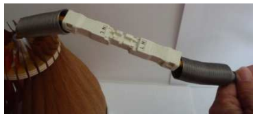
2- Insert the male connector into the female connector until you hear a "click"
